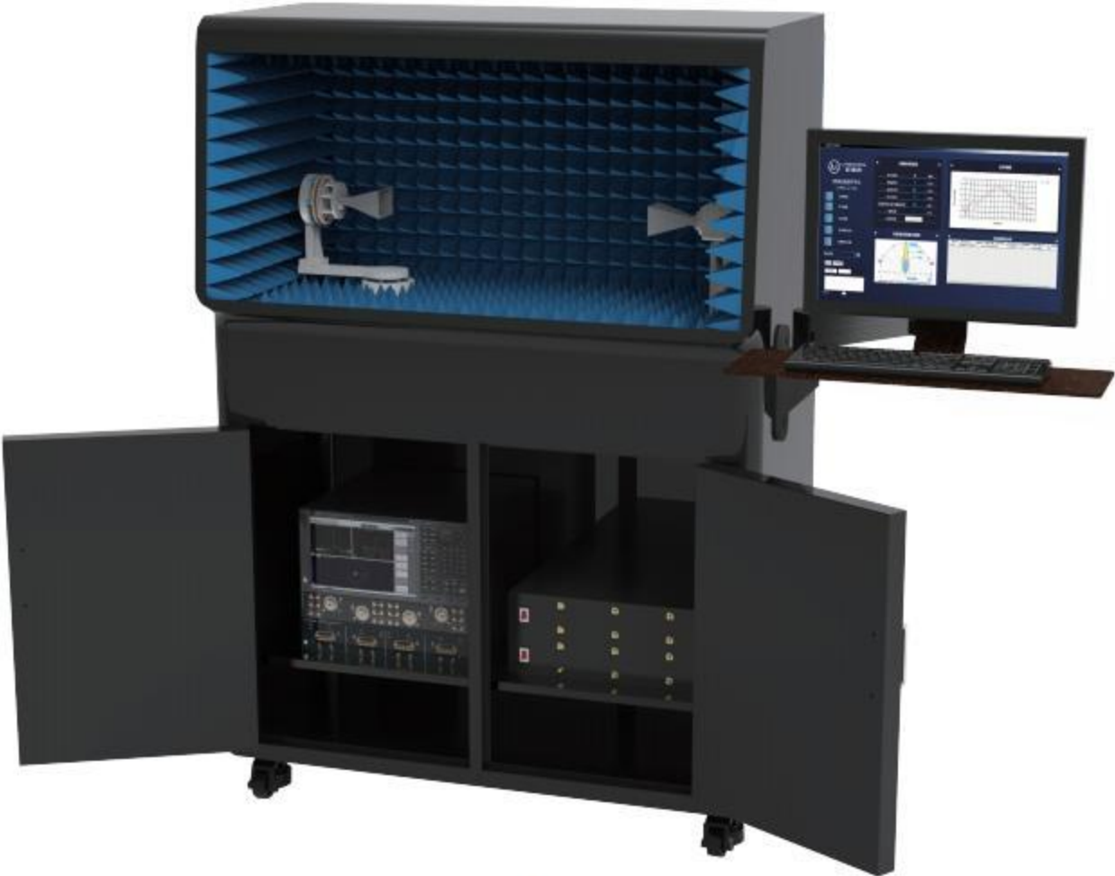
Desktop Version Teaching Solution Antenna Measurement Kit intergrating with a VNA, a set of antennas and RF cables, rotators and testing software.
